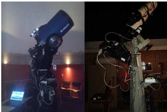
Fig. 3: Left: LHiRes III setup at 16" f/10 SC telescope at Dresden-Gönnsdorf observatory. Right: Setup at 180/1600 mm refractor at observatory Drebach.
